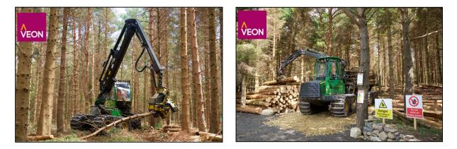
Photo 28 shows a harvesting machine felling a tree within a conifer stand. Photo 29 shows a forwarder stacking felled timber the roadside.
